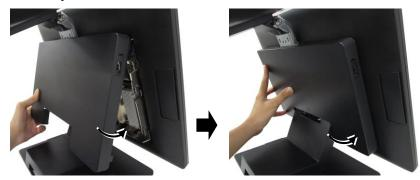
8. Install the dummy cover to the hinge bracket. Make sure the cover is hooked on the hinge bracket like below picture.
