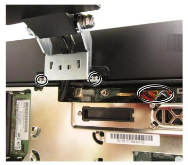
**For TM/LM-4011LVDS,** well insert the cable to the internal LVDS connector from the mainboard of **RT-1016A-G2** terminal, and tuck the extra cable inside the system compartment.
