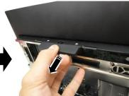
3. Remove the two countersunk head screws on both sides of the hinge cover.
