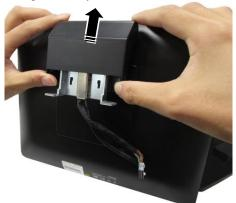
5. Lift the dummy cover a little and then remove it.
